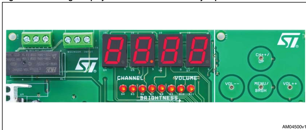
Figure 8. Message display when the MENU/BRGH key is pressed
