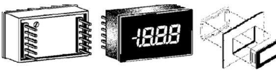
Splashproof, ultra low profile, 3½ digit snap-in meters with gasket. The SP Series can be front or rear panel mounted. 12 pin versions allow more modes of operation and compatibility with competing types. 8 pin versions are lower cost, easier to use and more suited to new designs
