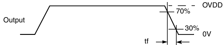
Figure 7. Definition of Timing for Standard and Fast-Mode
