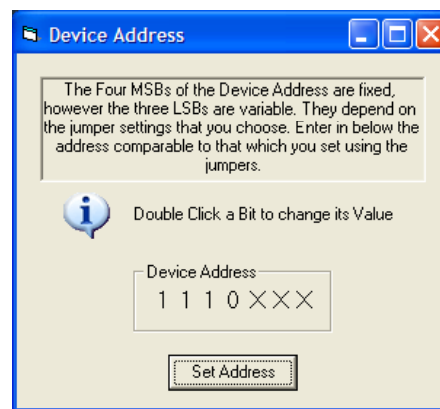
Figure 3. I 2 C Address Selection
