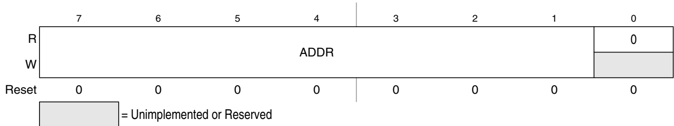
Figure 13-3. IIC Address Register (IIC1A)
