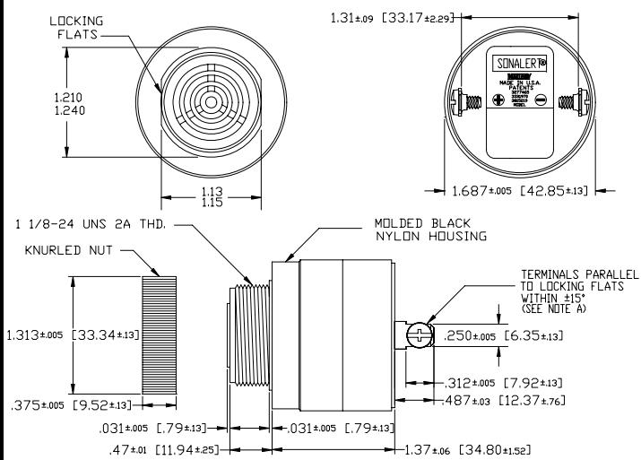
NOTE A: TERMINALS-.032 BRASS TIN PLATED, TAPPED FOR #6-32 SCREW, TWO #6-32 NICKEL PLATED BRASS SCREWS INCLUDED. WILL ACCEPT 1/4" QUICK CONNECT.
