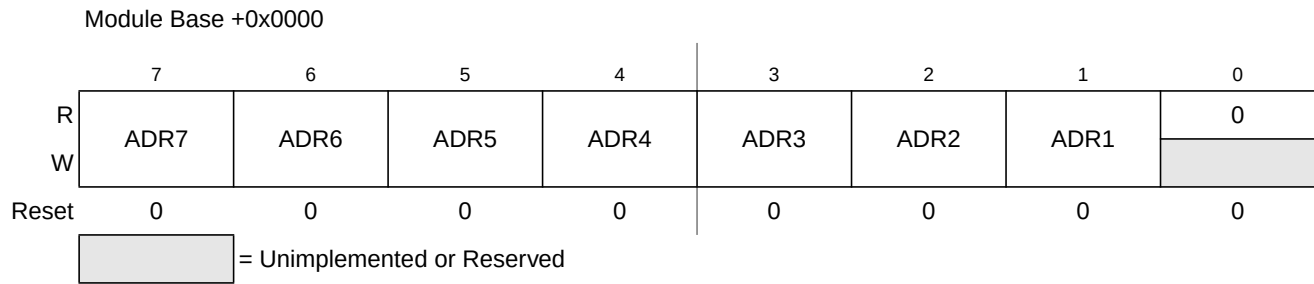
Figure 10-3. IIC Bus Address Register (IBAD)
