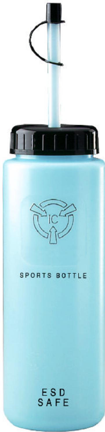
32-oz. static dissipative sports bottle for personal consumption of cold drinks. These bottles offer an average surface resistivity of  $10^9$  to  $10^{10}\Omega$  and can dissipate a  $\pm 5000V$  charge of in less than 2 seconds at 40% relative humidity.
