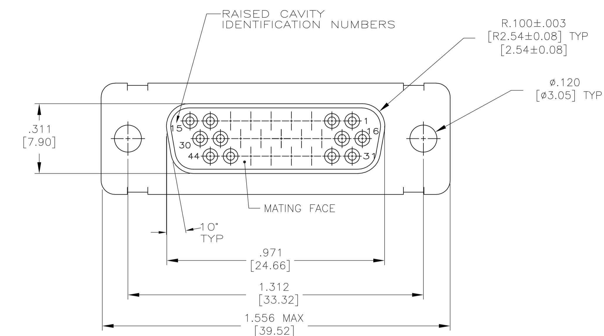
1. THIS RECEPTACLE WILL MATE WITH ANY 26 POSN, SIZE 2 PLUG IN AMPLIMITE SERIES.
