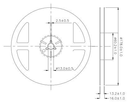
Note: The tolerances unless mentioned are ±0.1, unit=mm. Carrier Taping Dimensions: (Quantity: 1000PCS/Reel)
