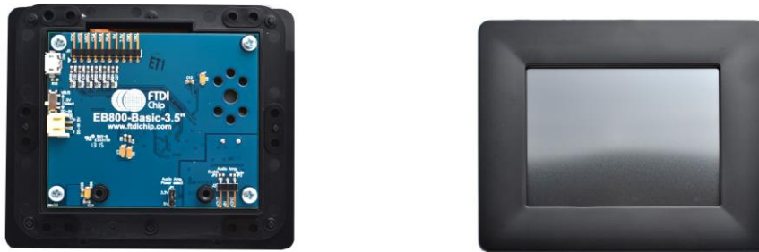
Figure 3-1 – VM800B module profile 3.5" display version
