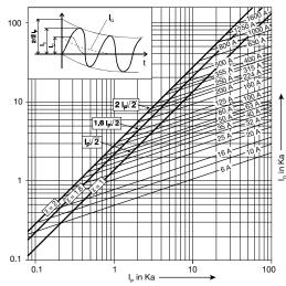
The prospective short circuit current is the value of the current, that would flow if there was no protection in the circuit.
