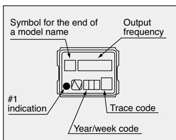
Because of space limitations, the output frequency is indicated as six digits including the decimal point.
