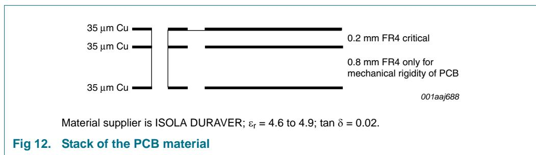
Fig 12. Stack of the PCB material
