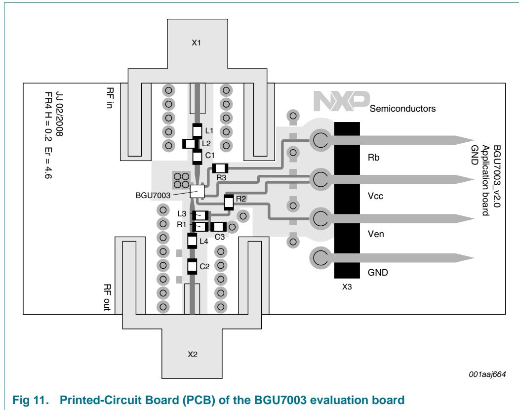
Fig 11. Printed-Circuit Board (PCB) of the BGU7003 evaluation board
