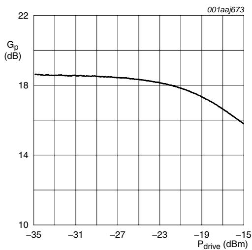
$T_{amb} = 25^{\circ}\text{C}$ ;  $V_{CC} = 2.5$  V;  $I_{CC(tot)} = 5.0$  mA;
