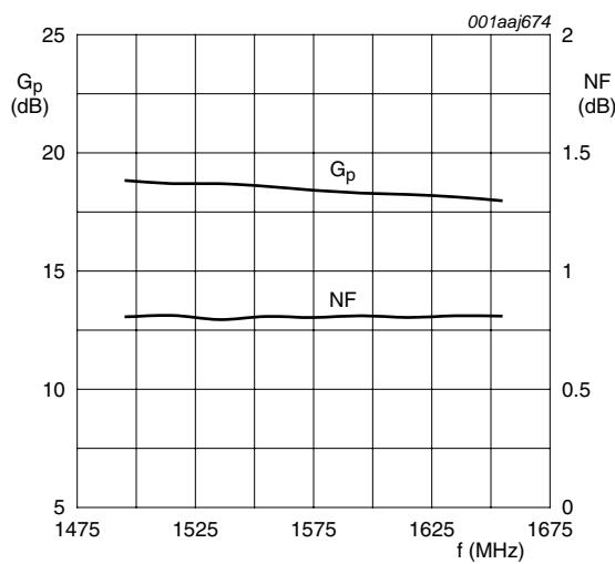
$T_{amb} = 25^{\circ}\text{C}$ ;  $V_{CC} = 2.5$  V;  $I_{CC(tot)} = 5.0$  mA;
