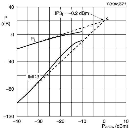
$T_{amb} = 25^{\circ}\text{C}$ ;  $V_{CC} = 2.5$  V;  $I_{CC(\text{tot})} = 5.0$  mA;
