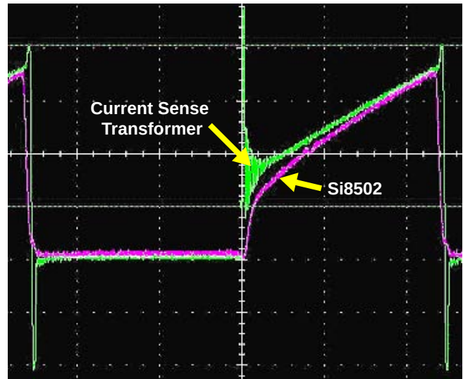
Figure 8. Leading-Edge Noise Suppression Waveforms (200 kHz, 9.3 A Load)
