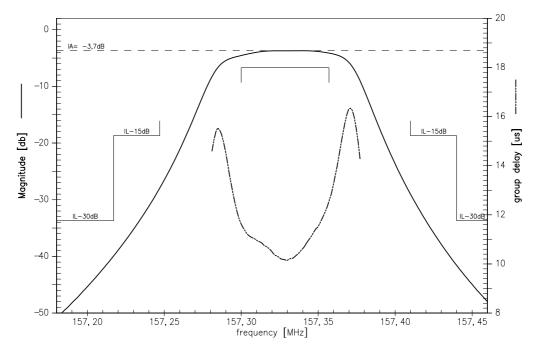
Transfer function wide band (measured unbalanced / unbalanced)
