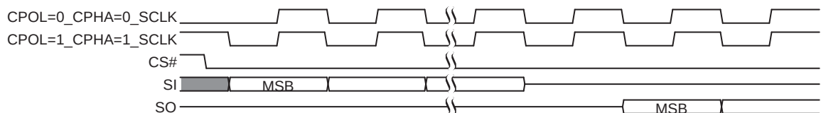
Figure 4.1 SPI SDR Modes Supported
