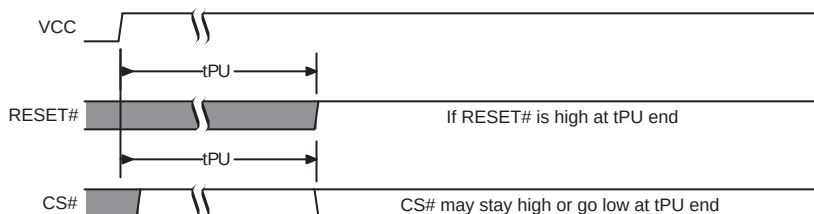
Figure 6.5 Reset High at the End of POR
