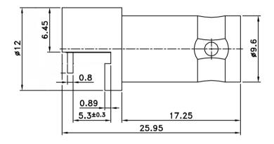
Body: Brass/Nickel Insulator: Teflon Pin: Brass/Gold
