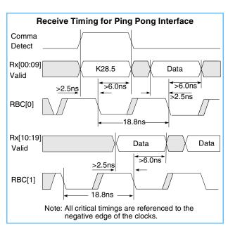
Rx[00:09] is timed off of RBC[0] as shown in the IBM42M10LCYAA20 portion of the OFC Timings on page 23. Rx[10:19] is timed off RBC[1] using identical timing specifications as in Receive Data (Rx[00:19]) on page 9. The skew between RBC[0] and RBC[1] shall not exceed  $\pm$  1.5ns.
