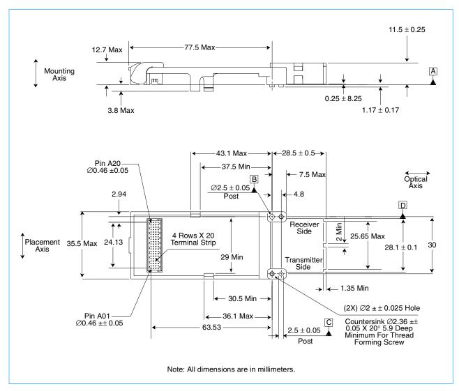
The transmit and receive circuits are electrically isolated on opposite sides of a double sided surface mount card. Two optical receptacles are at the end of the card. They are spaced 12.7mm apart to accept a standard duplex SC connector such as the one shown on page 27.
