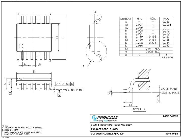
Note: For latest package info, please check: http://www.pericom.com/support/packaging/packaging-mechanicals-and-thermal-characteristics/
