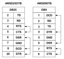
Loop back jumpers are pre-wired within the converter
