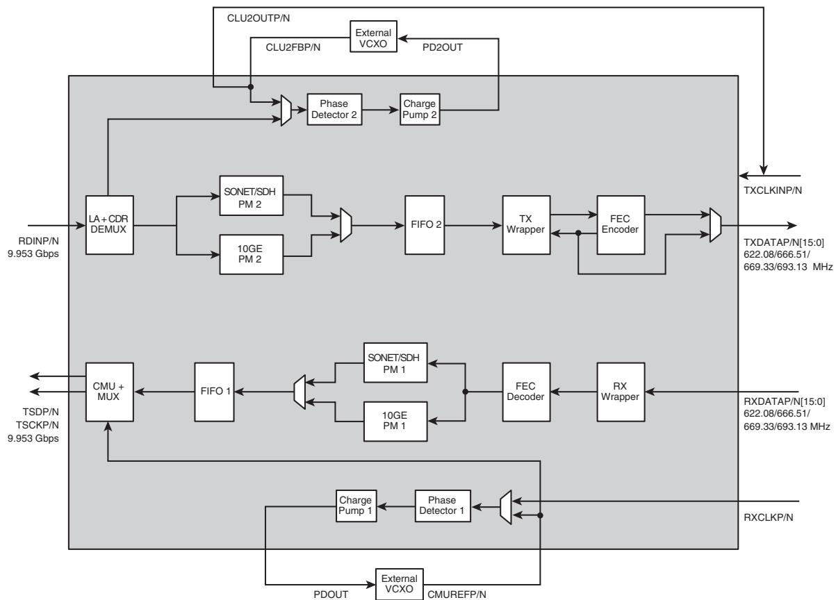
The BCM8512 is an 10 Gigabit DWDM transport processor that supports all the major functions on a DWDM line card:
