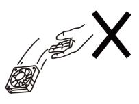
Don't cut the fan or lead wires
