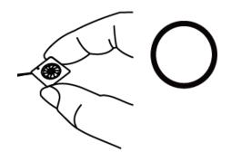
Don't pull fan with lead wires.
