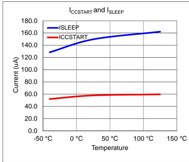
**Figure 10: Startup Current and Sleep Current vs. Temperature**
