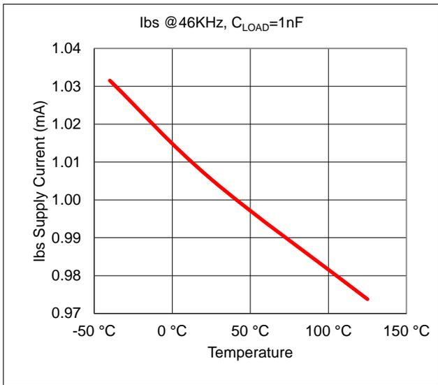
**Figure 13: I<sub>BS</sub> Current @1nF Load vs. Temperature**
