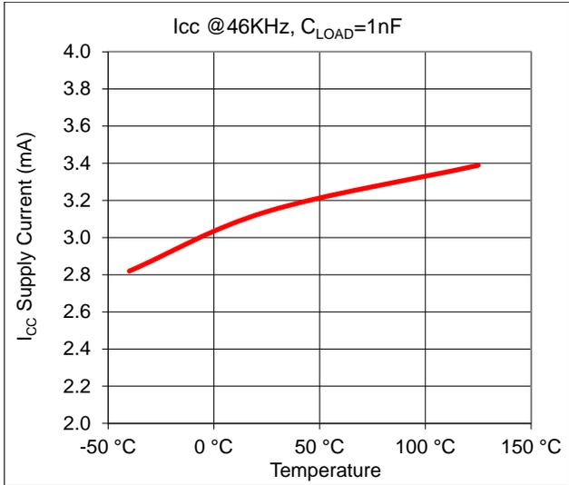
**Figure 11: I<sub>CC</sub> Supply Current @1nF Load vs. Temperature**
