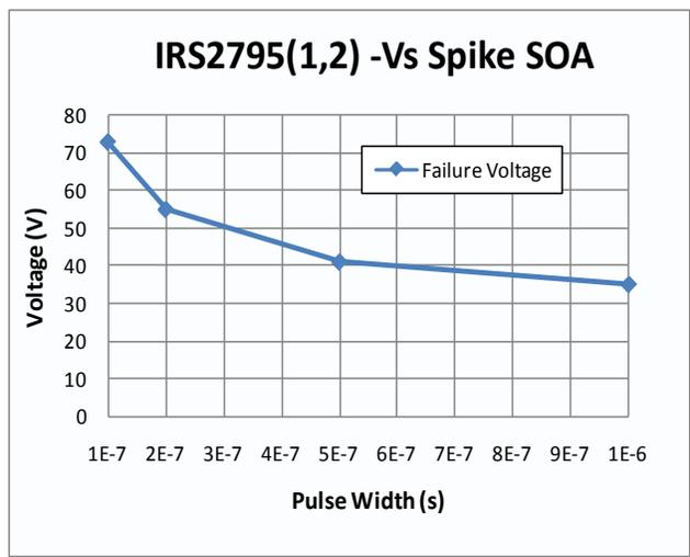
**Figure 18: VS Negative Transient Safety Operation Area**
