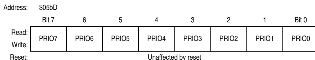
Figure 12-14. Transmit Buffer Priority Register (TBPR)
