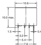
Note: Each value has a tolerance of  $\pm 0.3$  mm.
