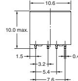
Note: Each value has a tolerance of  $\pm 0.3$  mm.
