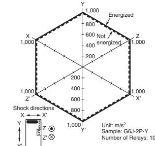
Conditions: Shock is applied in  $zx$ ,  $zy$ ,  $zx$  directions three times each with and without energizing the relays to check the number of contact malfunctions.
