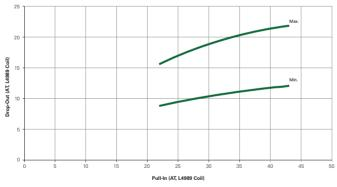
Note: Chart represents the range of Drop-Out, min to max for a given Pull-In value.
