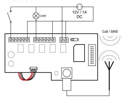
Call the configured STD35 with your mobile phone or send a SMS command and you can switch an electronic device which uses the connected power supply voltage.
