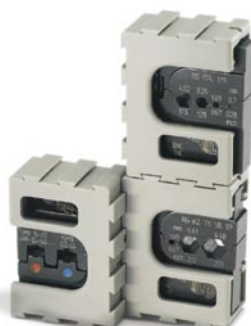
Crimp dies held together to facilitate storage in toolboxes.
