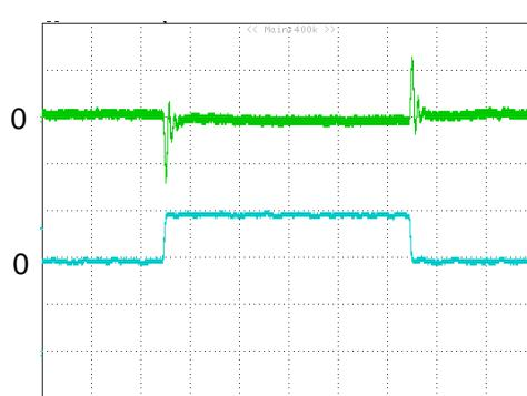
**Figure 9:** Output voltage response to step-change in load current (75%-50%-75% of  $I_o$ , max;  $di/dt = 1.0A/\mu s$ ). Load cap: 10μF tantalum capacitor and 1μF ceramic capacitor. Top Trace: Vout (100mV/div, 200μs/div), Bottom Trace:  $I_{out}$  (10A/div). Scope measurement should be made using a BNC cable (length shorter than 20 inches). Position the load between 51 mm to 76 mm (2 inches to 3 inches) from the module
