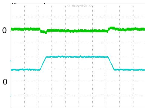
**Figure 8:** Output voltage response to step-change in load current (75%-50%-75% of  $I_o$ , max;  $di/dt = 0.1A/\mu s$ ). Load cap: 10μF tantalum capacitor and 1μF ceramic capacitor. Top Trace: Vout (100mV/div, 200μs/div), Bottom Trace:  $I_{out}$  (10A/div). Scope measurement should be made using a BNC cable (length shorter than 20 inches). Position the load between 51 mm to 76 mm (2 inches to 3 inches) from the module
