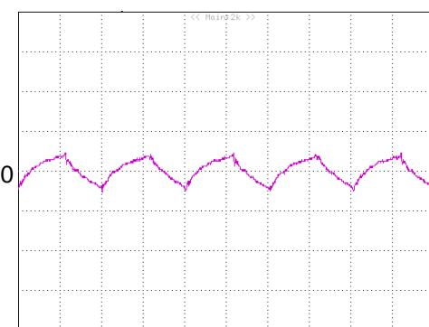
**Figure 14:** Output voltage ripple at nominal input voltage and rated load current ( $I_o=40A$ ) (100 mV/div, 1  $\mu$ s/div)
