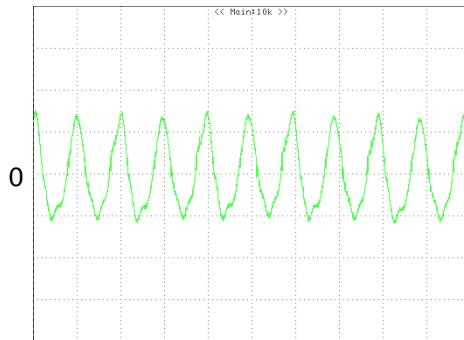
**Figure 11:** Input Terminal Ripple Current,  $i_c$ , at full rated output current and nominal input voltage with 12  $\mu$ H source impedance and 100  $\mu$ F electrolytic capacitor (100 mA/div, 2  $\mu$ s/div)
