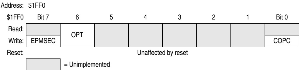
Figure 2-5. COP and Security Register (COPR)
