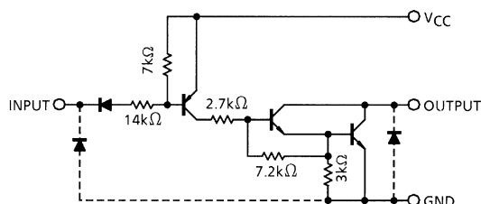
Note: The input and output parasitic diodes cannot be used as clamp diodes.
