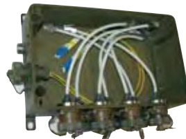
Kit with TVOP fiber connectors and RJFTV connectors
