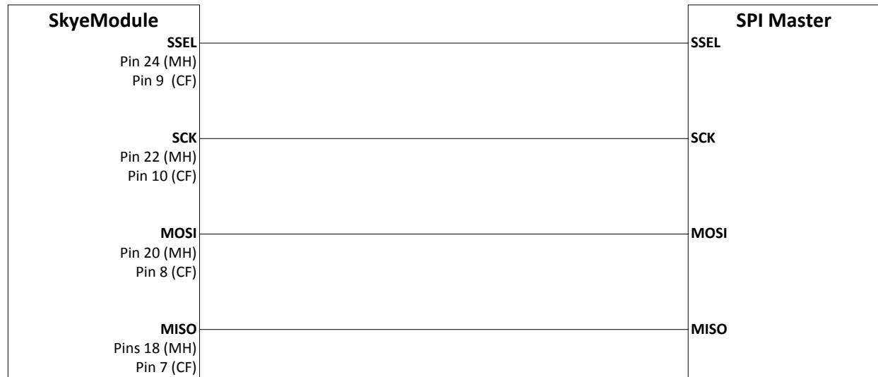
Figure 9-3: SPI Connection Diagram
