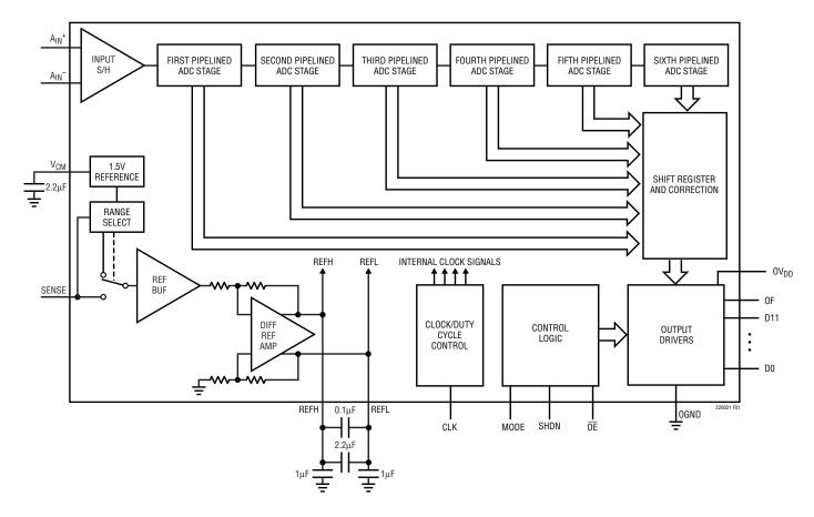
Figure 1. Functional Block Diagram (Only One Channel is Shown)
