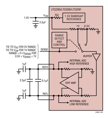
Figure 9. Equivalent Reference Circuit
