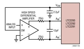
Figure 4. Differential Drive with an Amplifier
