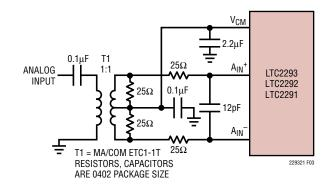
Figure 3. Single-Ended to Differential Conversion Using a Transformer
