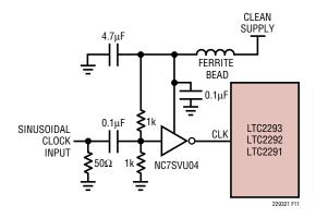
Figure 11. Sinusoidal Single-Ended CLK Drive
