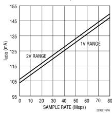
LTC2293: I<sub>OVDD</sub> vs Sample Rate, 5MHz Sine Wave Input, -1dB,
