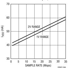
LTC2291: I<sub>OVDD</sub> vs Sample Rate, 5MHz Sine Wave Input, -1dB, O<sub>VDD</sub> = 1.8V
