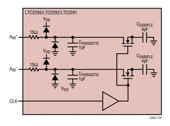
Figure 2. Equivalent Input Circuit
