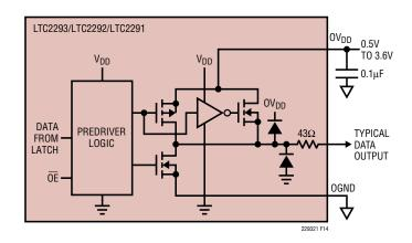
Figure 14. Digital Output Buffer
