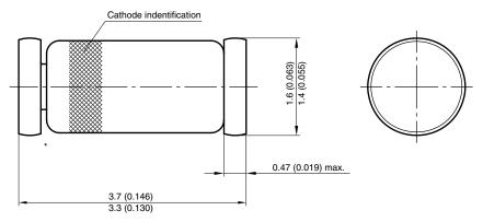
\* The gap between plug and glass can be either on cathode or anode side
