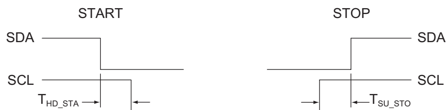
Figure 2: I²C Start and Stop Conditions;
