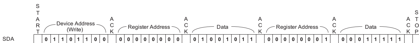
Figure 5: I 2 C Transfer Protocol for Example 1.
