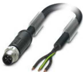
Power cable, 3-position, PVC, black, Plug straight M12 SPEEDCON, S-coded, on free cable end, cable length: 5 m, for AC current up to 16 A/230 V
