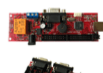
Olimex - SAM7-MT-256 DEVELOPMENT BOARD FOR AT91SAM7S256 ARM7TDMI-S MC >>
