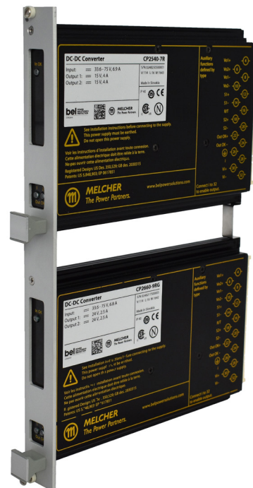
Front panel kit G05-6HE-Q01 (HZZ00838) accommodating two units for a 19" DIN-rack with 6 U, 5 TE.
