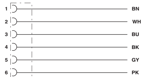
Contact assignment of M8 socket
