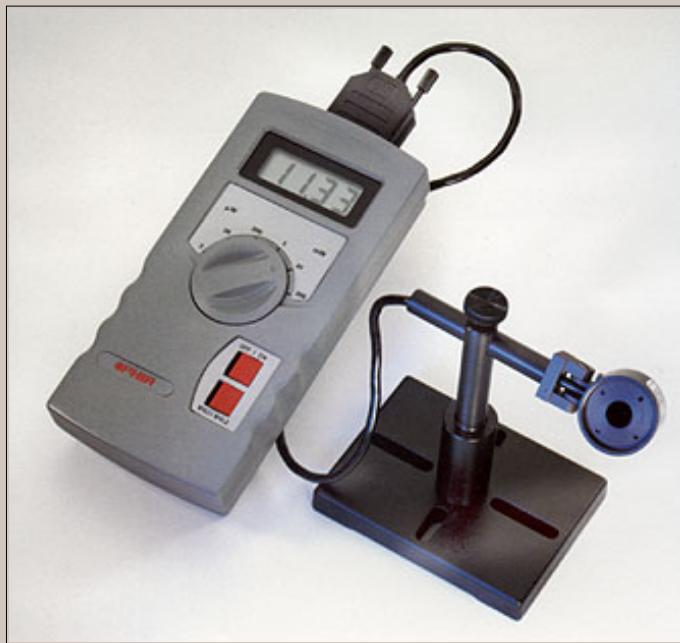
When you're working with laser diodes, you really should use an optical power meter – it's not just a matter of convenience.
