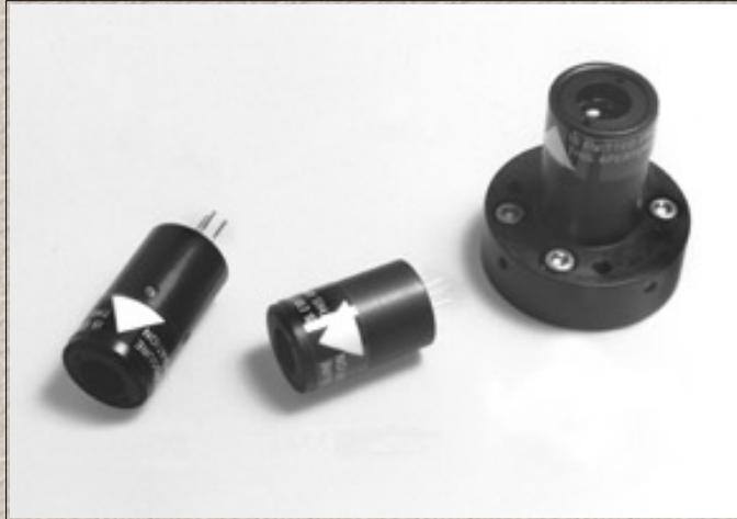
**What exactly is a Collimated Diode Laser?** A Collimated Diode Laser (CDL) is a compact cylindrical assembly often referred to as a light pen. Each CDL includes; a laser diode and collimating lens which are assembled into a precisely machined, black anodized, aluminum housing; the laser diode drive circuit is not included. CDL's are often a viable solution in the following situations:
