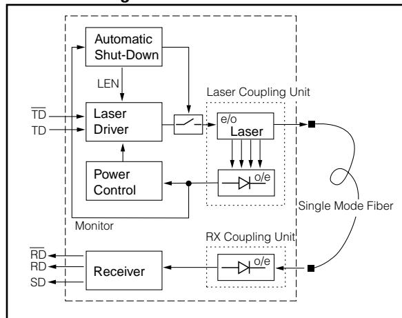
The receiver component converts the optical serial data into PECL compatible electrical data (RD and RDnot). The Signal Detect (SD, active high) shows whether an optical signal is present. If no optical input signal is present, the receiver data outputs are switched to static low level (RD=Low, RDnot=High).
