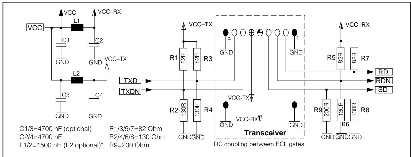
\*Recommended choke is Siemens Matsushita B78108-S1153-K or B78148-S1153-K ( $O_{min}=60$ , max. DC resistance=0.6 Ohm).
