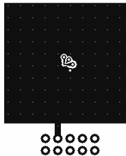
a. 65\text{ }^\circ\text{C/W} when mounted on a 1\text{ in}^2 pad of 2 oz copper.
