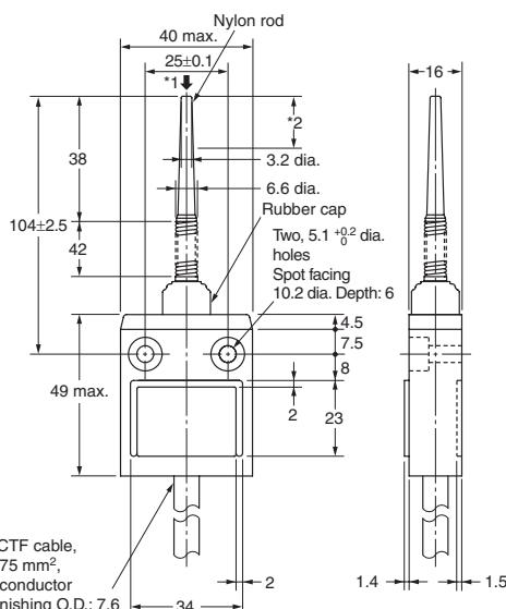
\*1 Operation is possible in any direction except in parallel to the axis.
