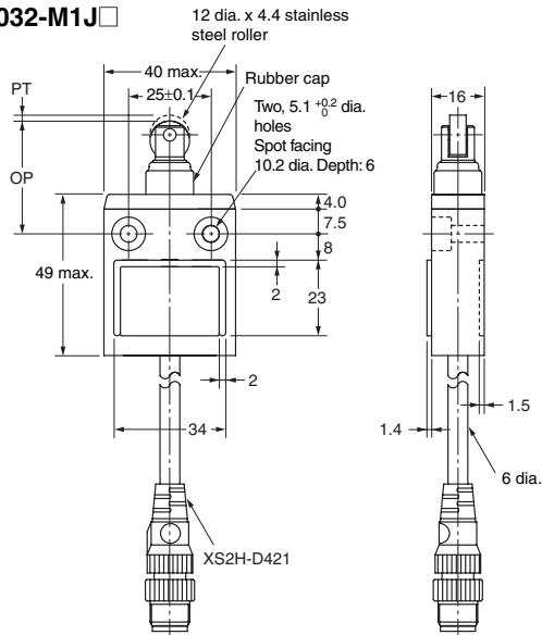
Note: Unless otherwise specified, a tolerance of ±0.4 mm applies to all dimensions.
