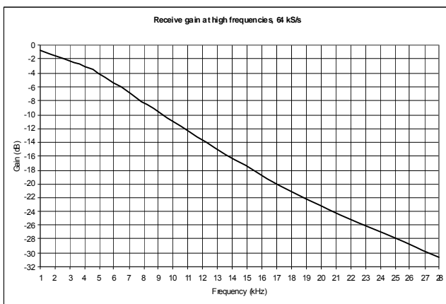
Figure 5. Receive Gain at High Frequencies (600 W)
