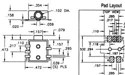
.088 (3) PLS Tape Spec's: 24mm wide; 16mm pitch CAT. NO. 982TR (Mono) Reel Spec's: 15 inch reel (1,000 pieces per reel)
