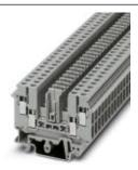
Disconnect terminal block, Connection type: Screw connection, Cross section: 0.2 mm² - 6 mm², AWG: 24 - 10, Nominal current: 16 A, Nominal voltage: 400 V, Length: 63.5 mm, Width: 6.2 mm, Color: gray, Assembly: NS 35/7,5, NS 35/15, NS 32
