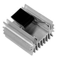
Ohmite's R2 Series (patent pending) heatsink provides a large surface area along with our C Series clipping mechanism to attach to a T0-220, T0-247, or T0-264 package. The self-aligning features of the clip assure secure attachment and enhanced thermal performance. Because no screws are required for device mounting, additional fins can be added to the rear side of the heatsink for increased total surface area in a more compact space.
