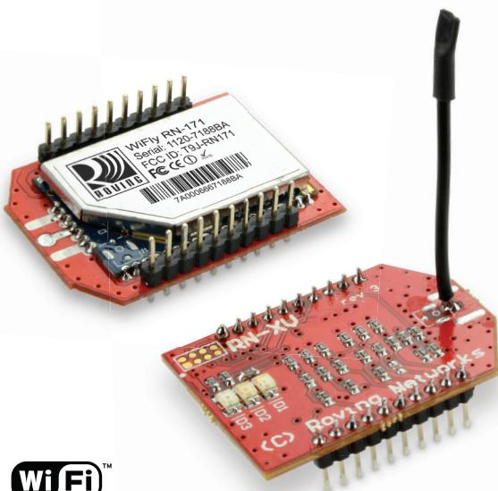
**The RNXV module by Roving Networks provides drop-in, certified Bluetooth or Wi-Fi™ connectivity for existing systems using 802.15.4 modules. Based on the popular 2 x 10 (2mm) socket footprint often found in embedded applications, the RNXV offers a complete wireless solution for customers looking to migrate to a standard protocol without modifying existing hardware.**
